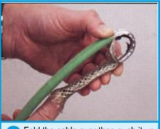
Fold the cable over then push it up 4 and out from the earth braid.
