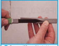
6 Remove 130mm of the inside jacket. Do not cut through the bus wires.
