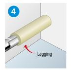
After installation of the trace heating cable, the pipes must be insulated with a minimum of 20mm lagging (Armaflex/PU Foam/Mineral Wool).
